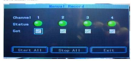
Select the cameras you want to record and start recording with START ALL. It is necessary that the user has the authority to start recording and an SD
