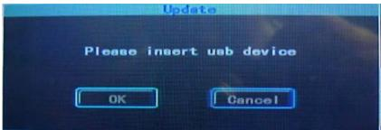
It 'also possible to an automatic update procedures by inserting the key and starting the DVR. In this way, if the system finds in stick a newer firmware
