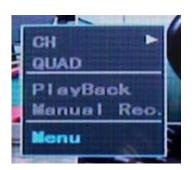
CH: You can select the full screen channels 1,2,3 or 4. The QUAD: Porta-screen multivision quad PlayBack: Access to the reproduction of recorded movies. Manual REC .: Starts manual recording Menu: Enters configuration
