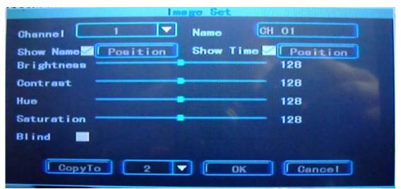
In this section you can adjust the video made by acting on the parameters of the image.
